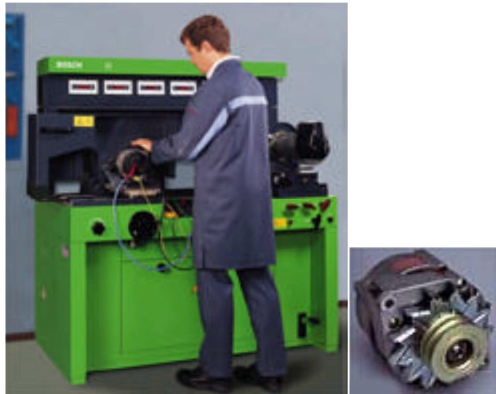
BOSCH component test stand with tested alternator
