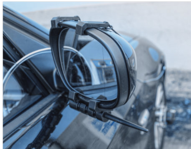
D x -antenna for mounting on side mirror
