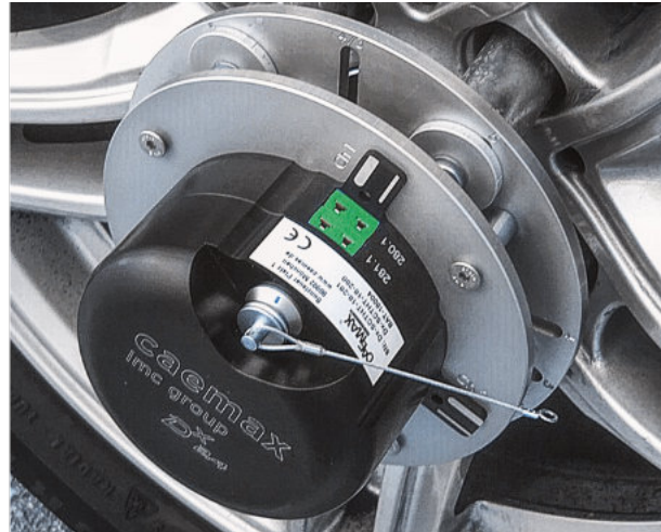
D x -transmitter module with 6 DI thermocouple channels type K
